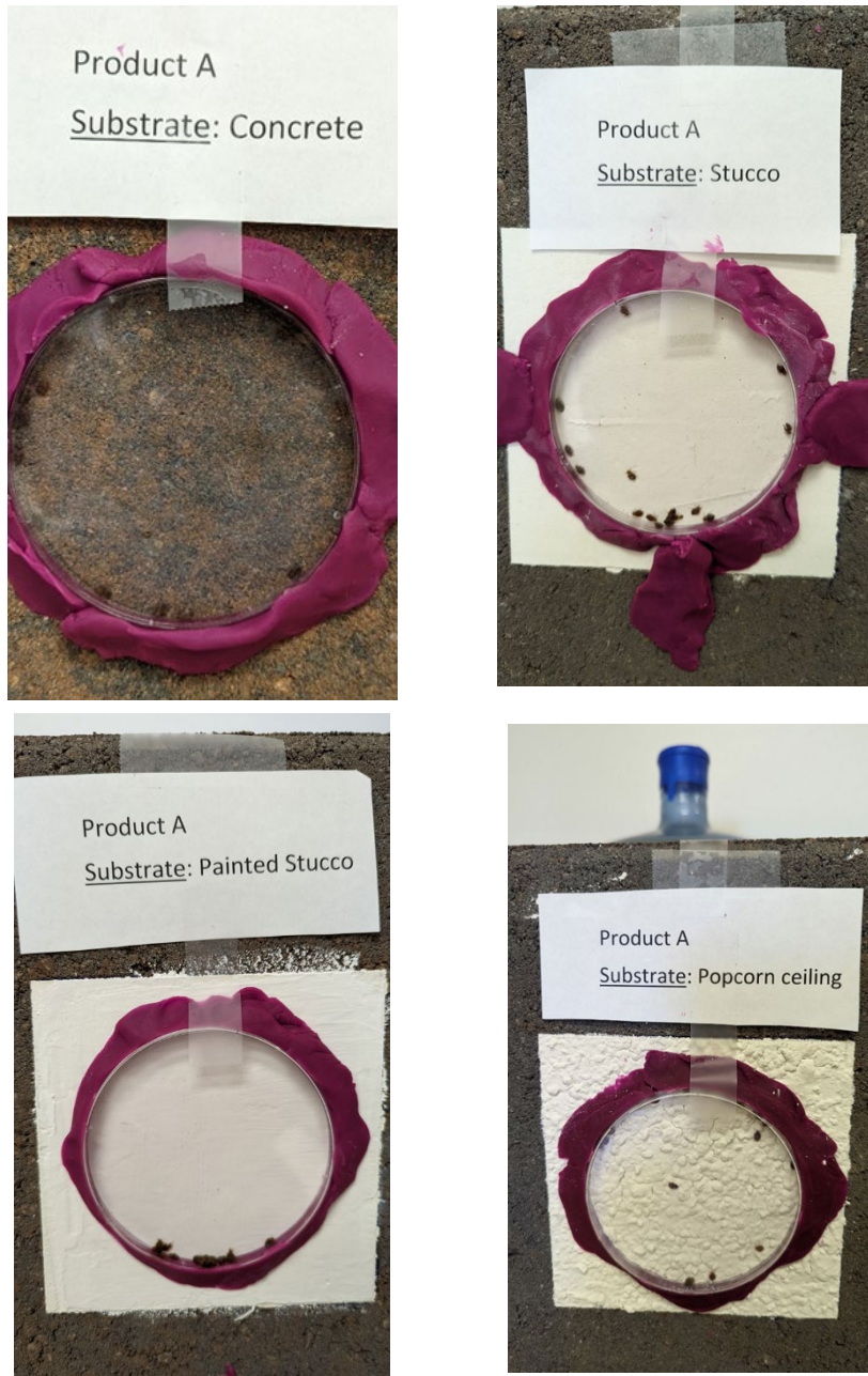
Figure 1. Surfaces that were treated with “CHINCHEX” for the forced exposure experiment with bed bugs. Squares of 12 x 12 cm were covered with one of the following coats stucco, painted stucco, or popcorn ceiling.
