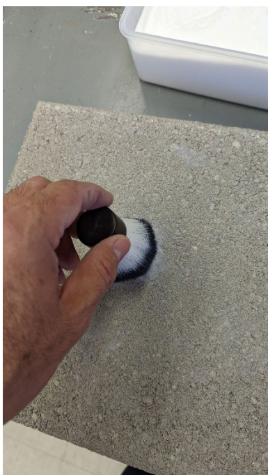
Figure 2. Makeup brush used for the application of “CHINCHEX” to concrete, stucco, painted stucco or popcorn ceiling.
