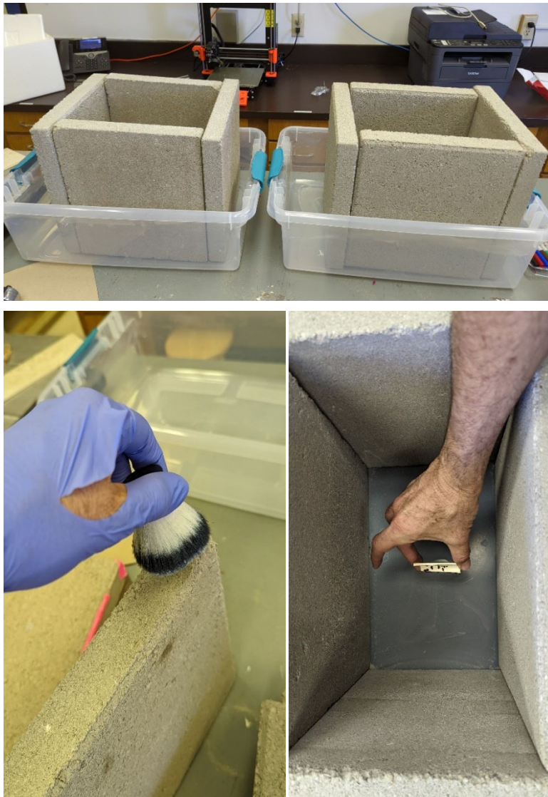
Figure 3. Above, Concrete blocks assembled to form crevices, common bed bug refuges; left , application of “CHINCHEX” to external edges of blocks with a makeup brush. After assembling, these edges will conform the bed bug harborages; right , bed bugs harboring in a paper tent which was placed in the center of the blocks.
